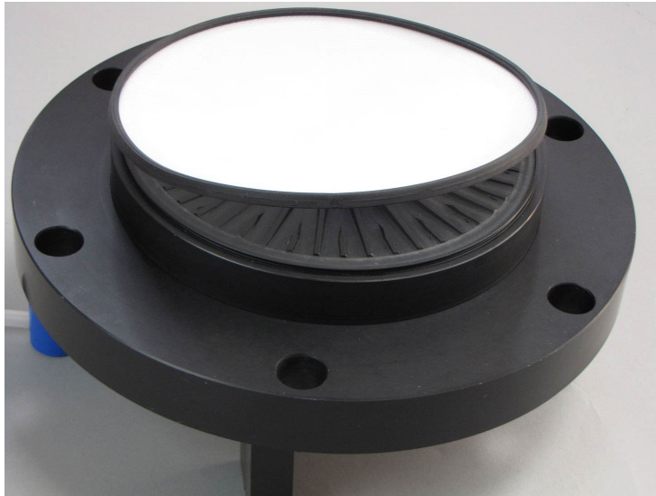
Figure 8: Photograph showing the installation of the fixed bed support.
